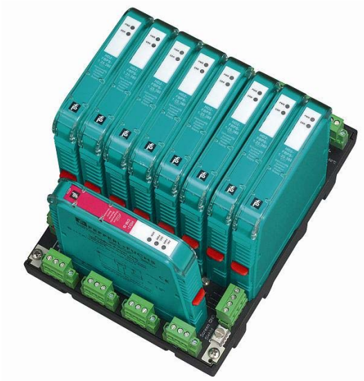
Fig. 3: Fieldbus power supply with integrated Advanced Diagnostic Module for the physical layer. Special connections adapted to control technology enable simple plug and play functionality.
